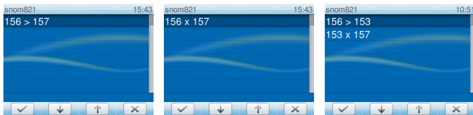
Monitored extension ringing Monitored extension busy Simultaneous calls
